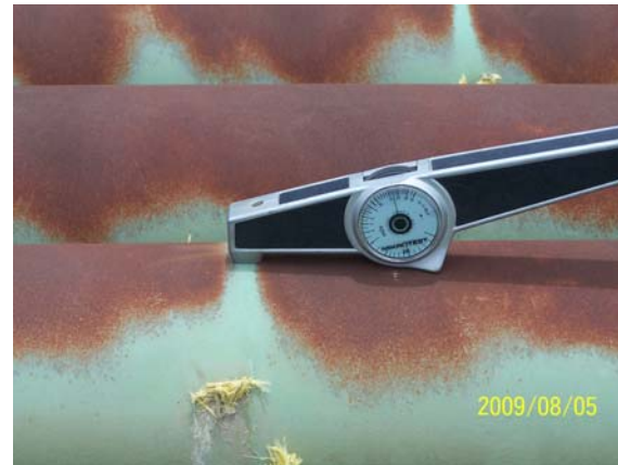
Thickness of UV Protected Area (17 mils)
