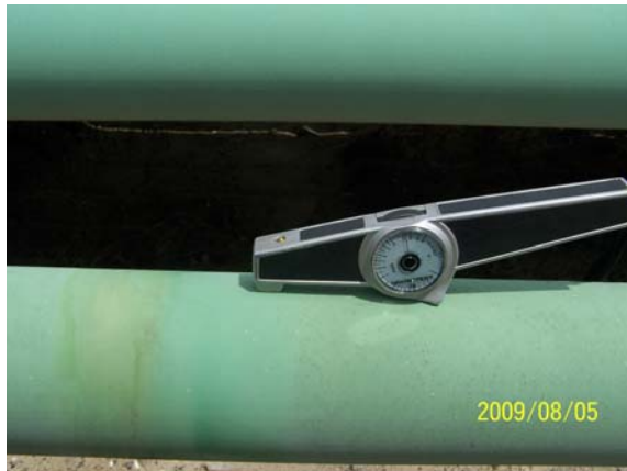
Thickness of UV Exposed Area (16.5 mils)
