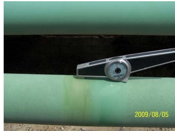
Thickness of UV Protected Area (17.5 mils)
