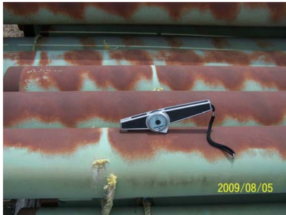
Thickness of UV Exposed Area (3.7 mils)
